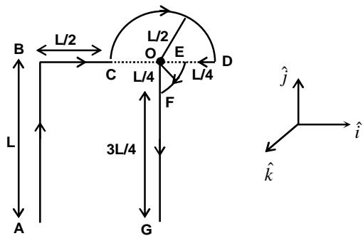
$$\vec{B}_{\text{Net}} = \vec{B}_{AB} + \vec{B}_{BC} + \vec{B}_{CD} + \vec{B}_{DE} + \vec{B}_{EF} + \vec{B}_{FG}$$
